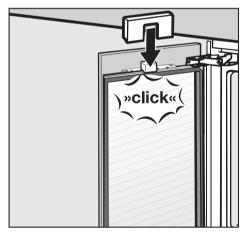
Fit the cover to the light contact switch so that it clicks into place as shown.
